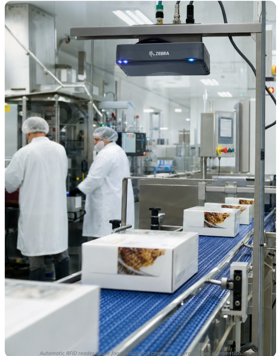
Automatic RFID reader above food production conveyor — zero manual intervention.
